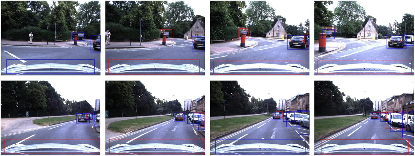
Fig. 6. Sample vehicle tracking results: each row indicates the tracking results in continuous frames. Blue boxes: detected vehicles. Red boxes: tracked vehicles. As can be seen, missing detection can be successfully tracked.
