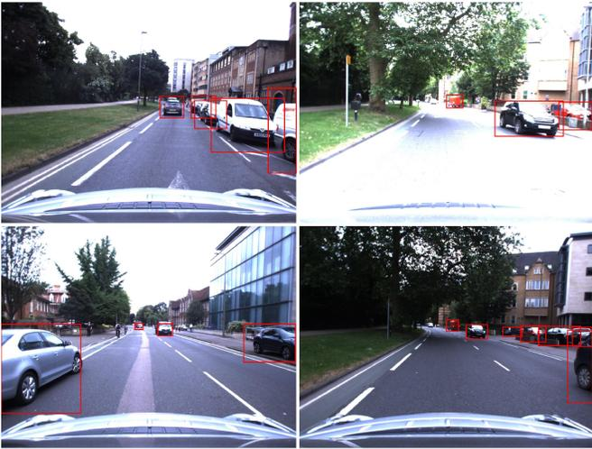
Fig. 5. Sample vehicle detection results from our YVDN on Oxford RobotCar Dataset. Red boxes: detected vehicles. As we can see, the detector is robust to occlusion and illumination.
