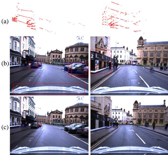
Fig. 7. Examples of vehicle removal from each laser scan. Each column represents an example vehicle removal pipeline. (a) Single laser scan frame; (b) Laser points projection to image and vehicle detection and tracking on image; (c) Vehicle points removal for vehicle-free laser scan.
